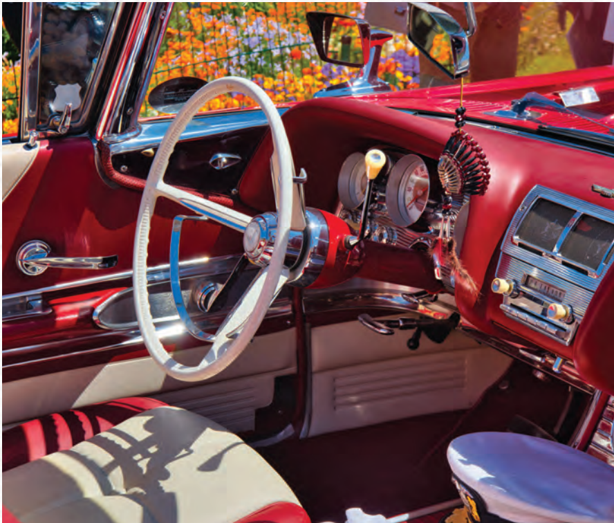
A three-on-the-tree gear shift (with a white knob on the end) in a Thunderbird on show at a meeting in Baden-Baden, Germany in 2022.
