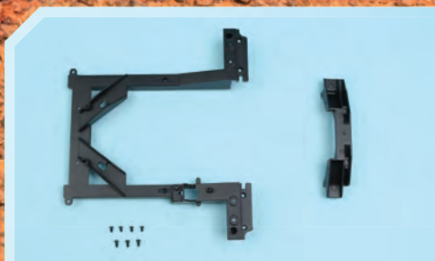
Chassis Frame and Crosspiece
