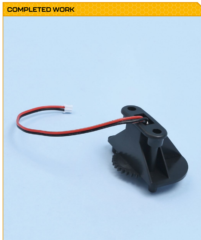
#01-COMPLETED WORK A motor has been fitted inside its housing and a cog has been attached.
