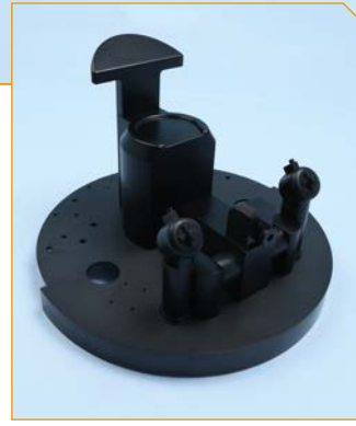
#018-11 Fit the video stand assembly from step 9 on to the base assembly from step 3: the side supports 18F and 18H 'hug' the columns 17C and 17D ; screw sockets on the base of parts 18H , 18D and 18F align with screw holes in the base 17E (circled).
