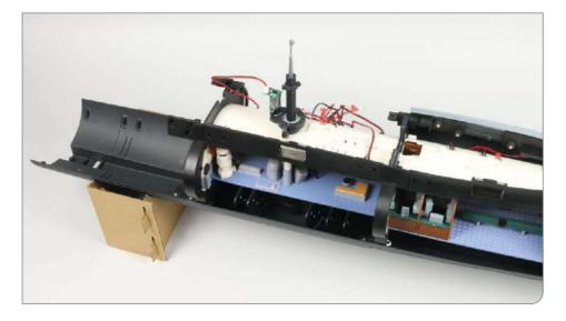
Two connectors and a magnet (fixed onto a mounting plate) have now been added to the hull assembly. Note: keep any spare screws safely aside.
