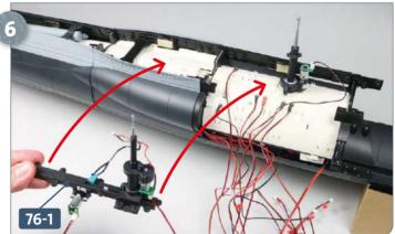
Place your model on your work surface. Position the navigation periscope assembly on top of the deckheads of the second and third compartments, as indicated by the arrows.
