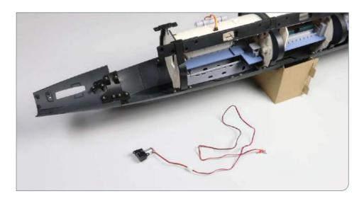
The motor of the port (L) side propeller has now been inserted into housing and connected to a cable. Another piece of housing has also been attached to the main assembly. The motor itself will be installed in the next kit.
