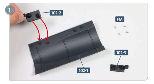
Firstly, place the port (L) hull plate **102-1** (outside facing down), connector **102-2**, connector **102-3** and four **FM** screws on your work surface. Take the connector **102-2** and fit it onto the raised sockets on the hull plate, as indicated by the arrows.
